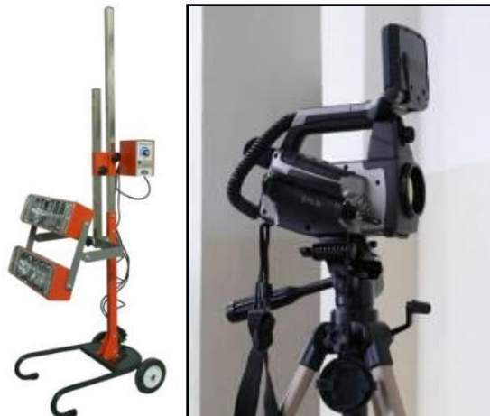
Figure 4. Equipment used in examinations: infrared radiators type FOBO EP 102 and FLIR ThermaCAM P65 thermal camera.
